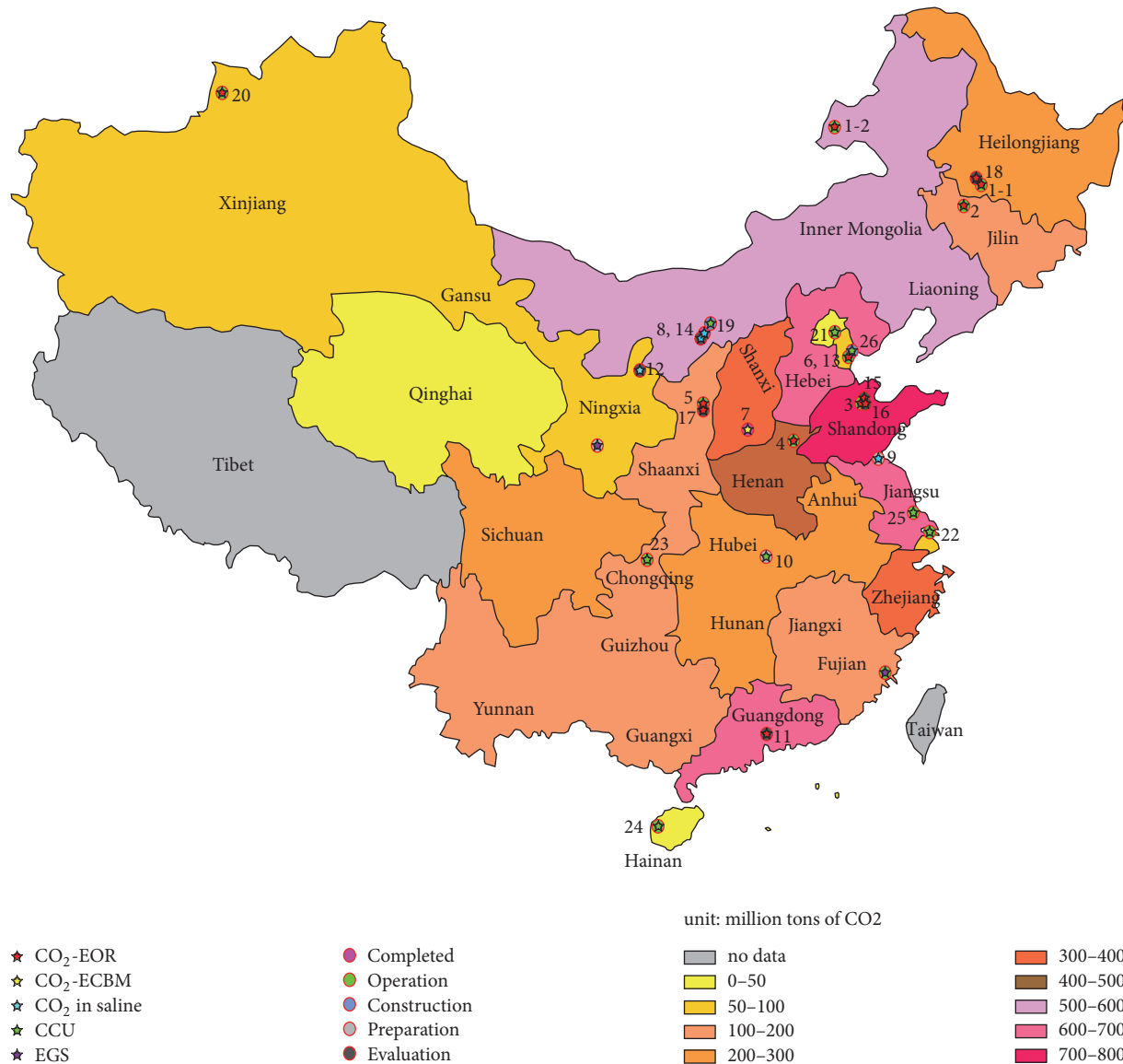
FIGURE 7: Distribution of CCUS engineering projects in China excluding the South China Sea Islands (numbers defined in Table 3) superimposed on the provincial CO 2 emission map for the year 2010 (from [34]).
